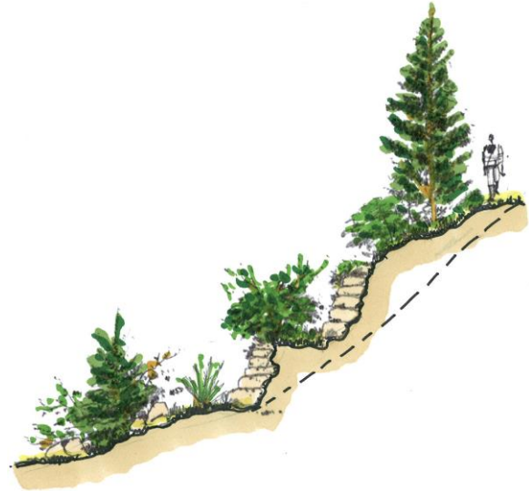
Figure 3 – Stepped Retaining Structures with Planter
